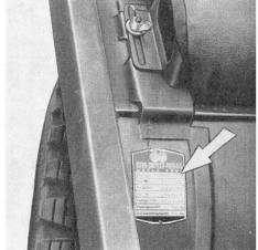
Older Haflingers (early 60s) have the type plate mounted in a slightly different position.
