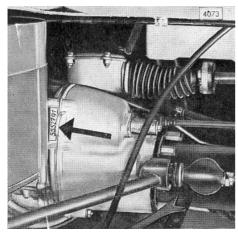
The **chassis number** is also stamped onto the right side of the gearbox housing.
