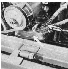
The **engine number** is also stamped onto the engine crankcase, close to the oil dipstick.
